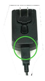
**2D)** Plug the other end of the USB-C cable into the power supply.
