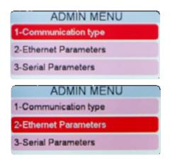
**2E)** Select "Ethernet Parameters", then "IP Configuration", then "DHCP activation" and then select "Off" and press the green "Enter" key.
