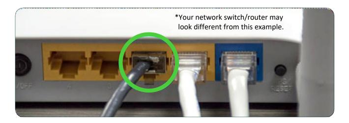
**2B)** Connect Lane/3000 power supply to 120V power outlet and to the back of the Lane/3000 Ethernet cable. *Note: Lane/3000 will turn on once connected to power.*
